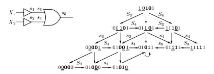
**Fig. 2.** Circuit  $C_2$  and its binary analysis
