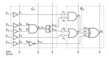
Fig. 4. Sample circuit with partition.
