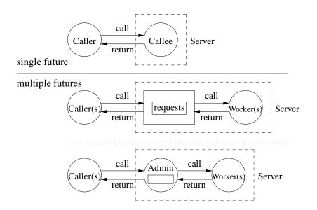
Figure 3.3: Basic Server Structures
