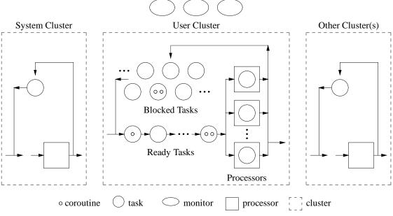
Figure 2.1: Runtime Structure of a  $\mu$ C++ Program
