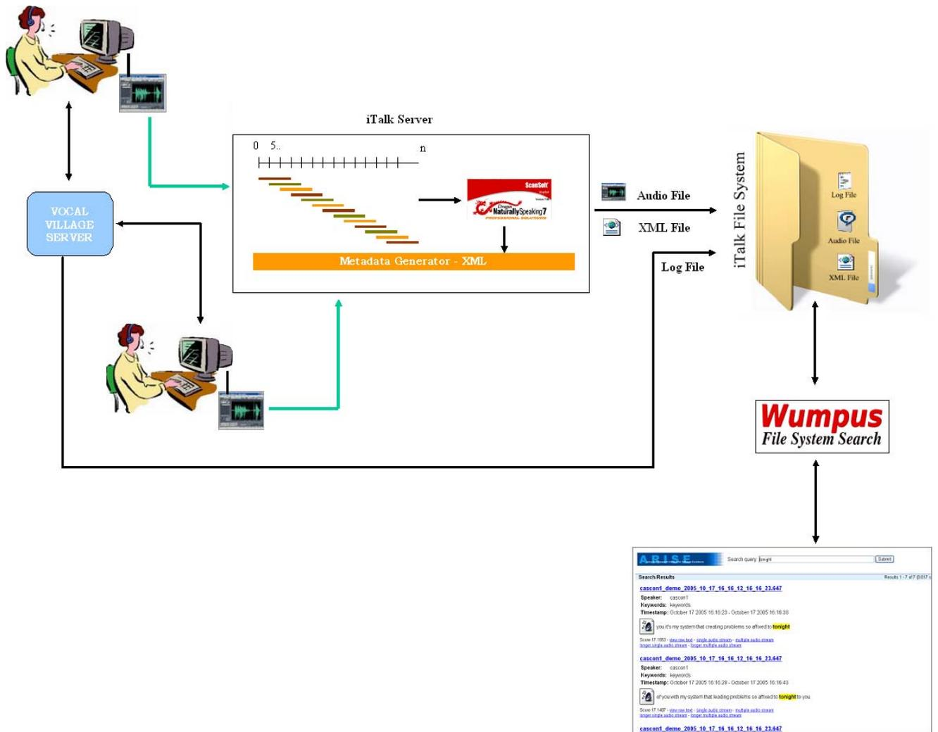
Figure 25: Detailed iTalk server architecture
